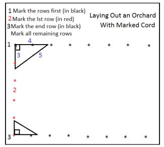
lay out an orchard is with a surveyor's transit and compass or laser guidance system. For do-it-your-selfers, the next best way is to prepare a cord or rope with markers (e.g. colored tape) each distance the rows will be apart. Mark a second rope with the tree spacing distance marked on to be used at right angles to the line of rows. For 40' x 40' spacing, a second marked rope is not necessary. DO NOT USE NYLON CORD - it has too much "give." Binoculars would be useful to ensure straight lines.
